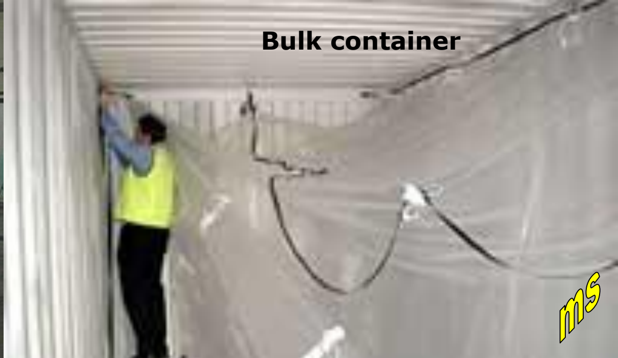
Open top bulk liners can be fitted to either open top containers or bulk containers.
